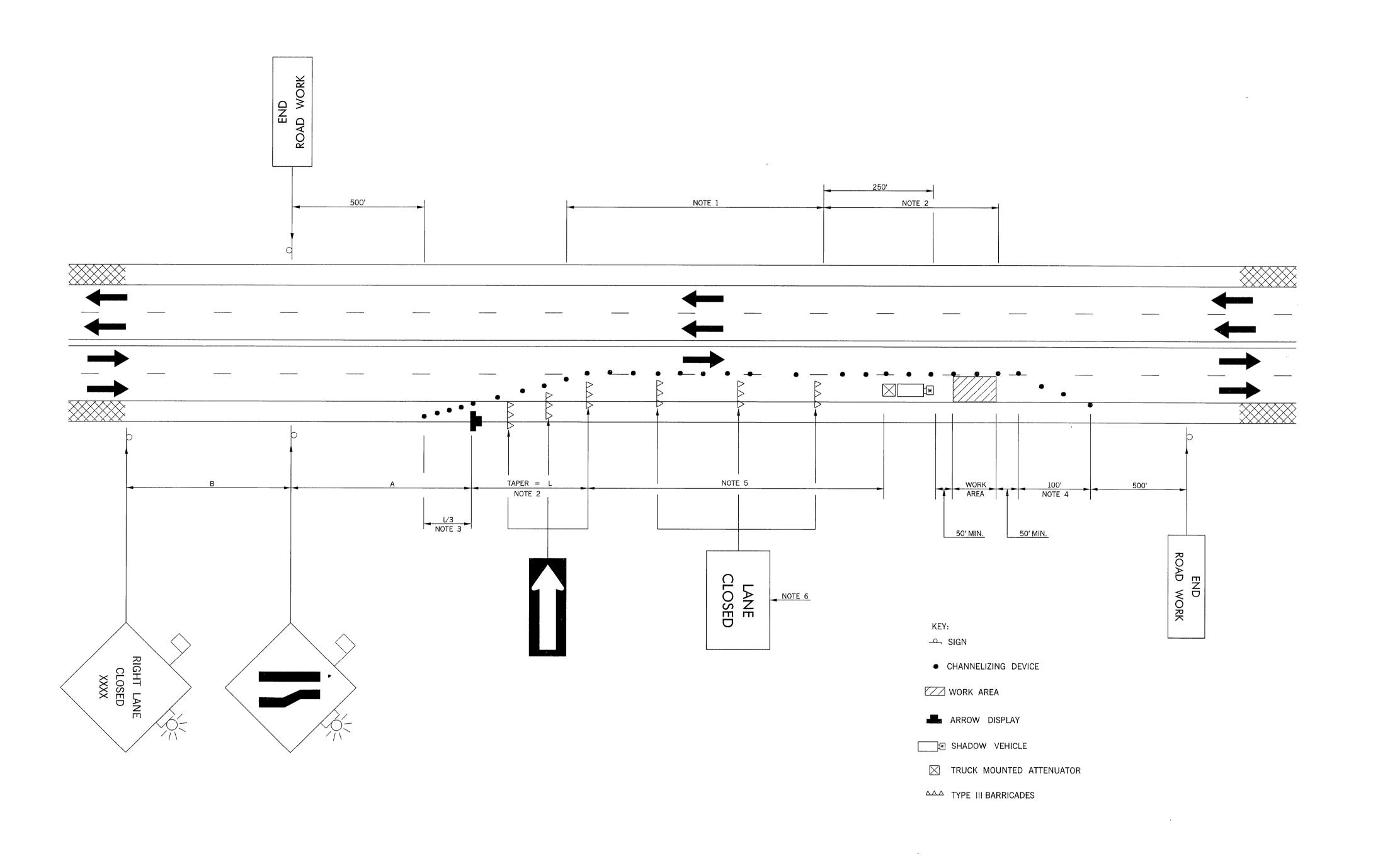
MAXIMUM SPACING OF CHANNELIZING DEVICES SHALL BE AS FOLLOWS: (A) FIRST 250 FEET OF ACTIVITY AREA.
