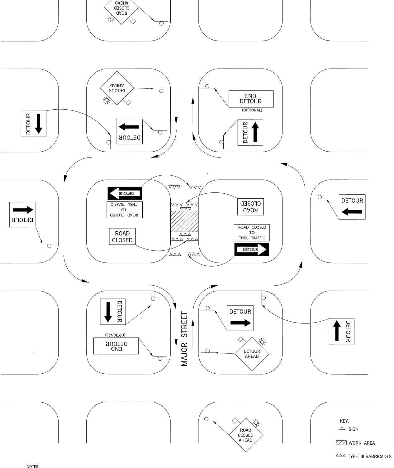
NOTES: WARNING LIGHTS SHOULD BE USED TO MARK BARRICADES AT NIGHT AS NEEDED.
