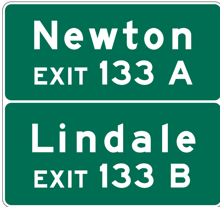
Figure 2E-17. Supplemental Guide Signs for Multi-exit Interchanges
