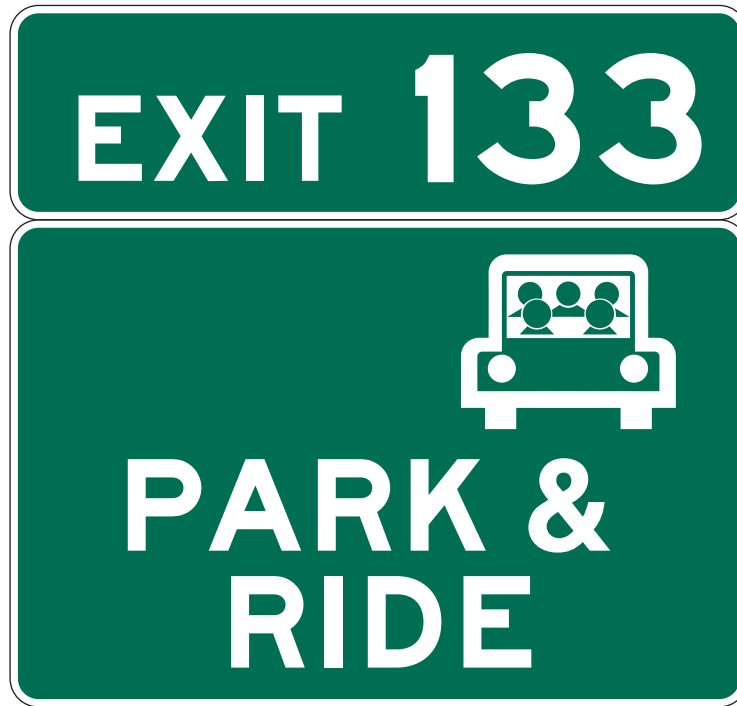
Figure 2E-19. Supplemental Guide Sign for a Park and Ride Facility (Route with Exit Numbering)
