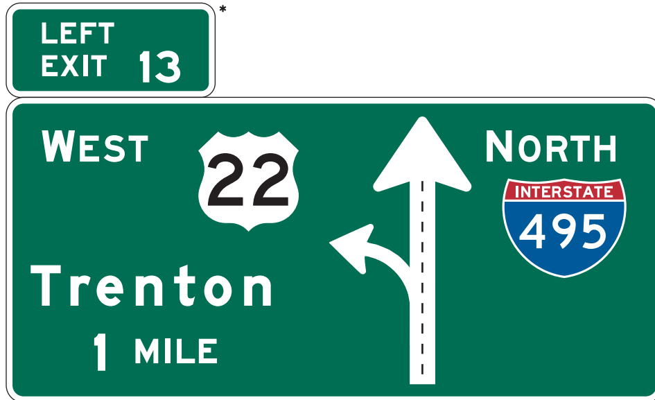
Figure 2E-3. Diagrammatic Sign for a Single-Lane Left Exit
