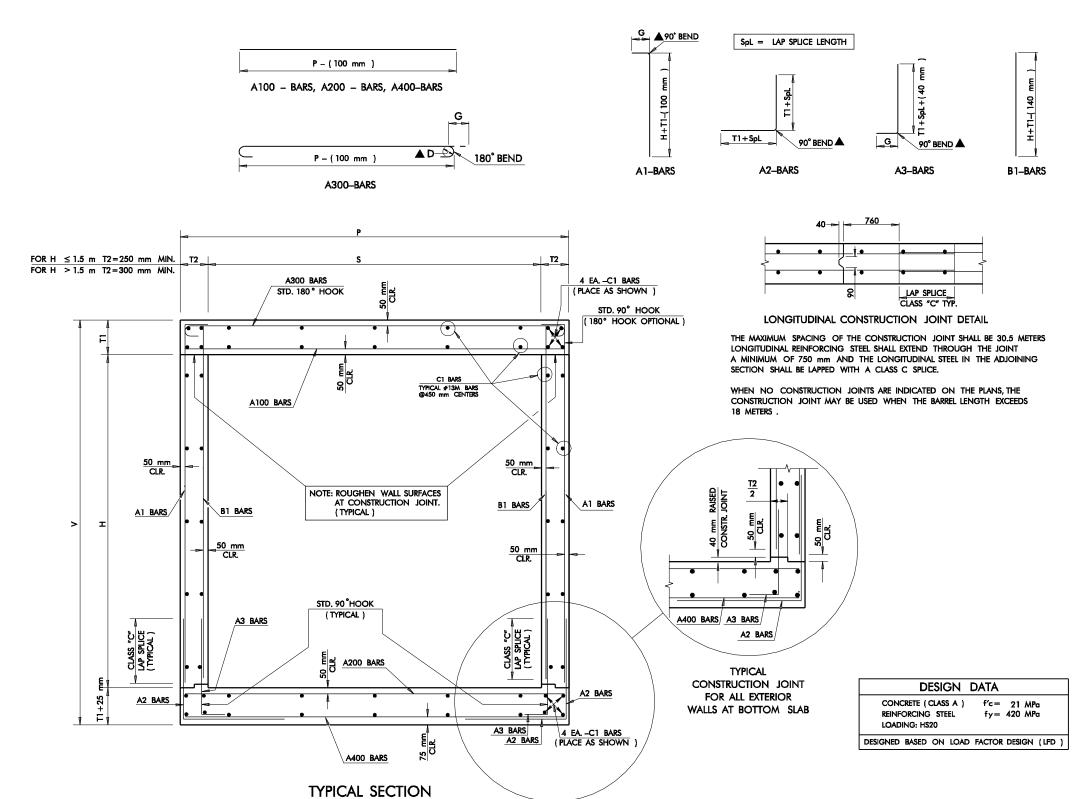
SINGLE CELL REINFORCED CONCRETE BOX CULVERT
