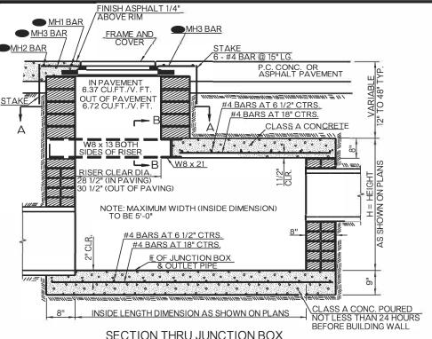
SECTION THRU JUNCTION BOX (SHOWN IN PAVING WITH RISER)
