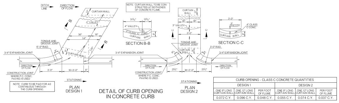
ALL QUANTITIES SHOWN IN THIS TABLE ARE BASED ON WIDTHS SHOWN FOR EACH DESIGN, AND ARE FOR ONE 12" LONG CURTAIN WALL, ONE 9" LONG CURTAIN WALL AND PER FT OF FLUME LENGTH.
