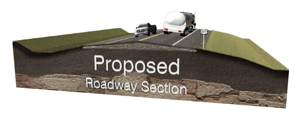
Proposed US-277 TYPICAL SECTION TWO (2) 12' DRIVING LANES and 8' SHOULDERS on Each Side
