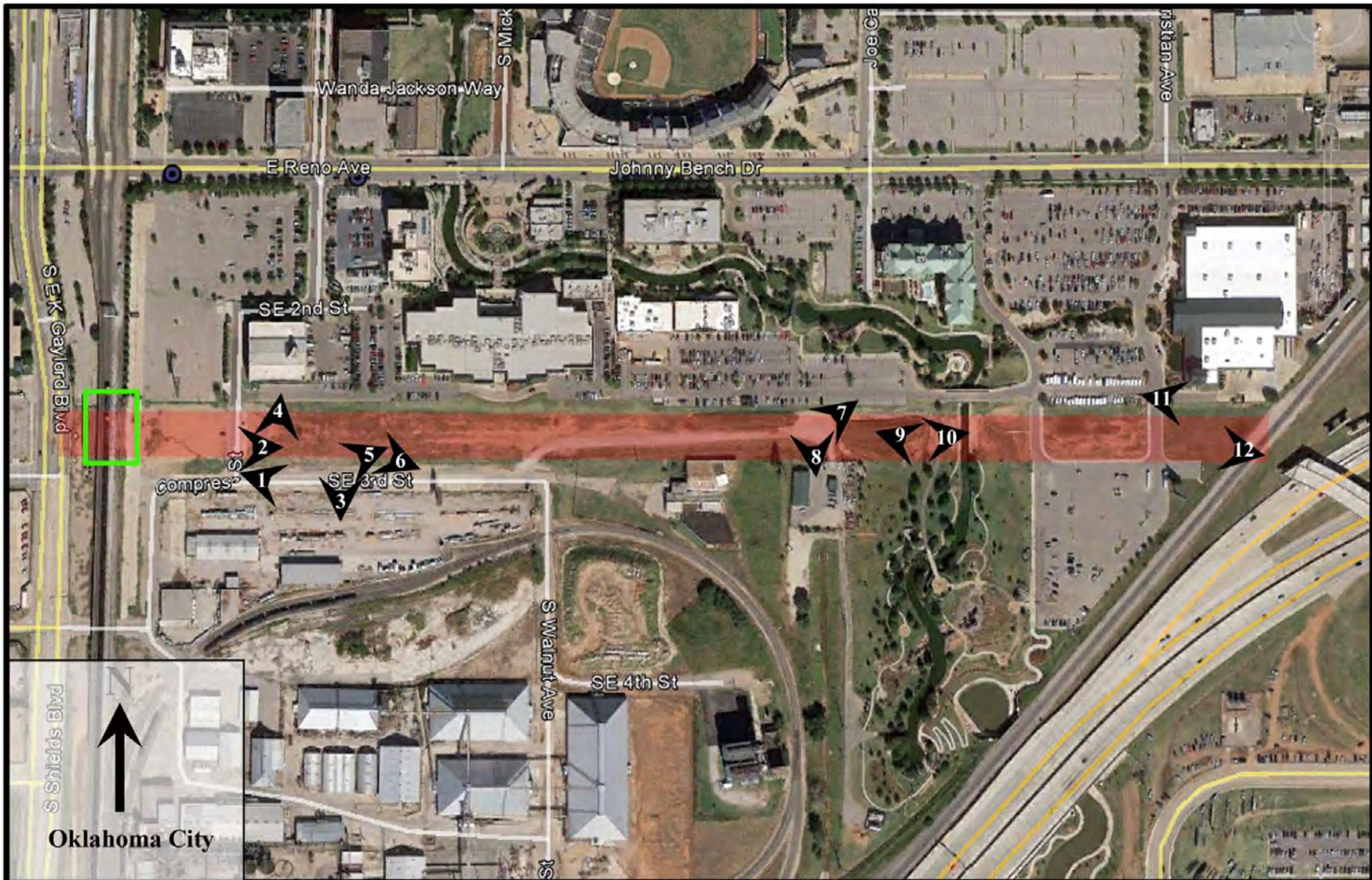
Figure 2. Proposed Crosstown Boulevard tie-in along previous I-40 corridor from E.K Gaylord, east to highway interchange. Note proposed underpass illustrated in green graphic.
