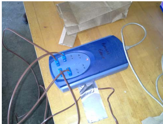
Figure 12: Photograph of the TC-08 data logger for temperature monitoring.
