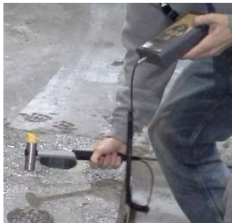
Figure 9: Photograph of the Nitto hammer in use.
