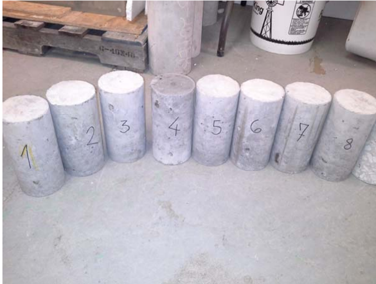
Figure 7: Photograph of eight in-place cylinders of one of the slabs.
