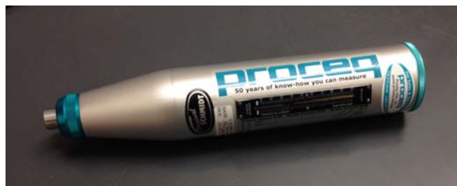
Figure 8: Photograph of the rebound hammer.
