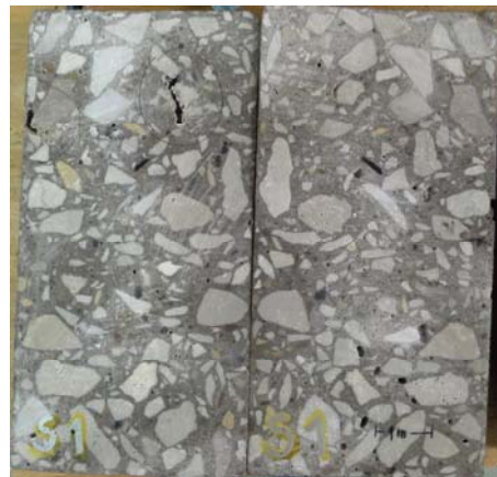
Figure C.1e: Sleeve vibrated cylinder 1 sawed
