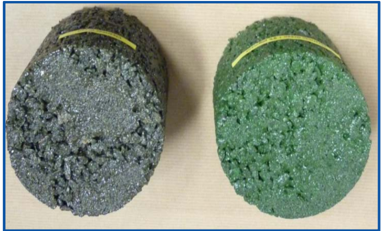
Figure 21. Asphalt without pigment (left) and asphalt with green pigment (right)
