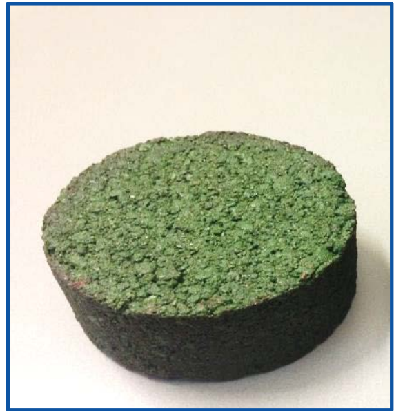
Figure 24. Asphalt Concrete sample topped with thin layer of green pigmented asphalt
