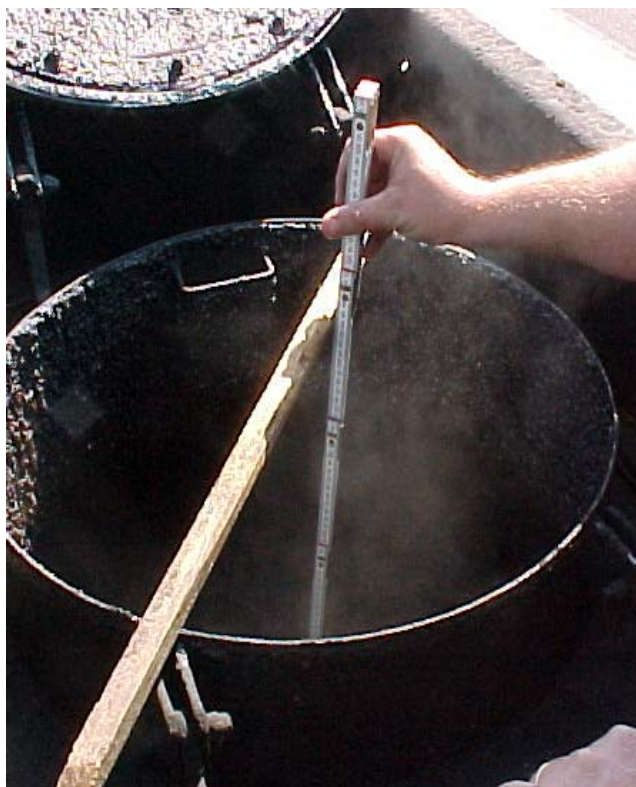
Figure 1 - Measure tank level (Note that safety precautions were not used in this photo. Always wear safety protection equipment for this operation)
