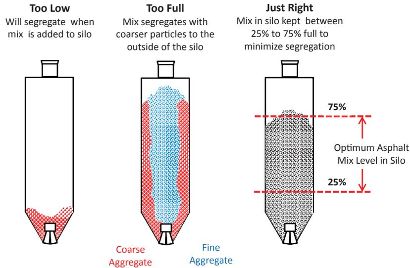
FIGURE 44 Schematic of storage silos with different volumes of mix [Source: Brock et al. (2003); Stroup-Gardiner after Murphy (2012a)].
