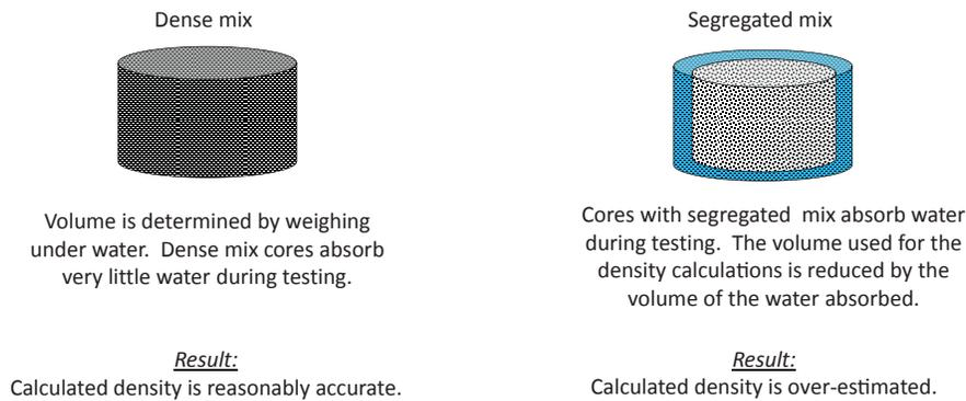
Successful laboratory density testing of segregated mix uses samples which are coated on the outside so water can't be absorbed.
