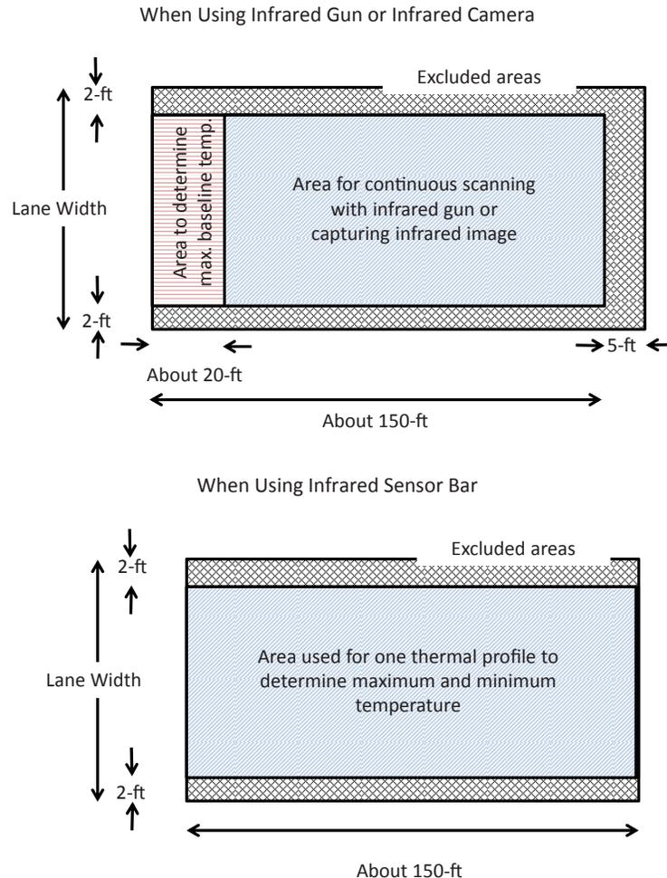
FIGURE 66 Area specified for one thermal profile [Source: Tex-244-F (TxDOT) (2014)].
