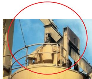
FIGURE 43 Proper use of bin charging batcher over silo [Source: Stroup-Gardiner after Murphy (2012a)].
