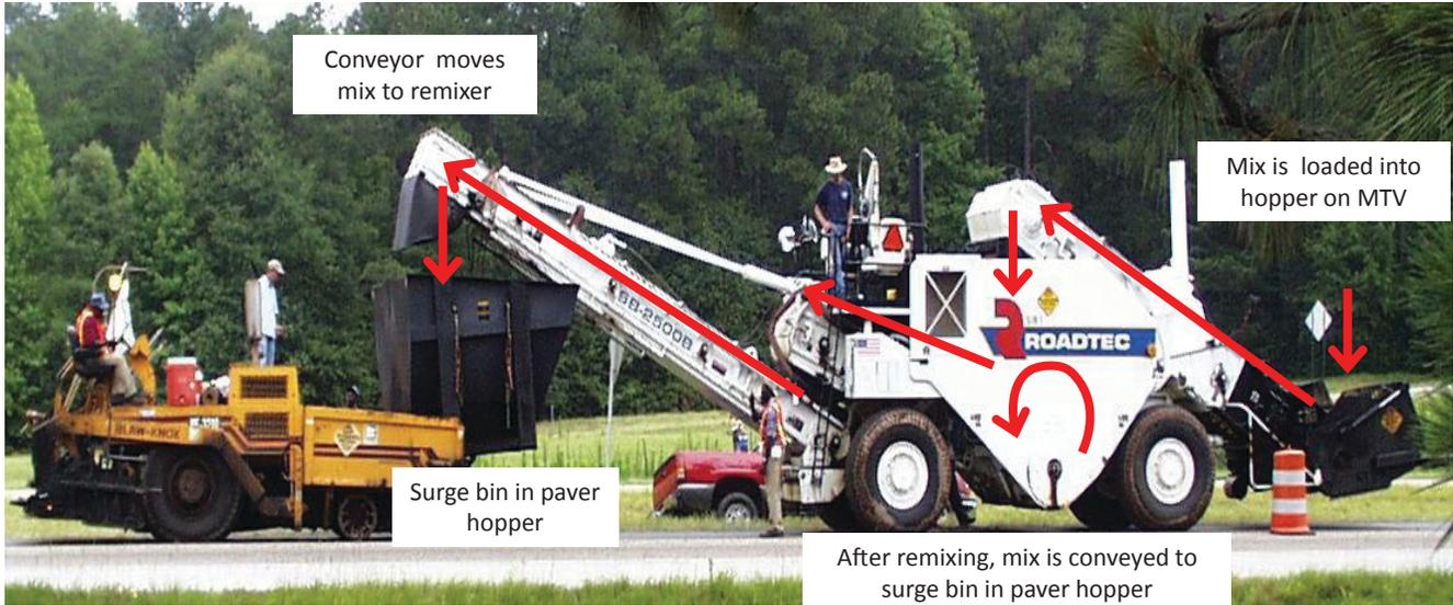
FIGURE 55 Example of remixer as a separate unit [Source: Stroup-Gardiner (2014)].
