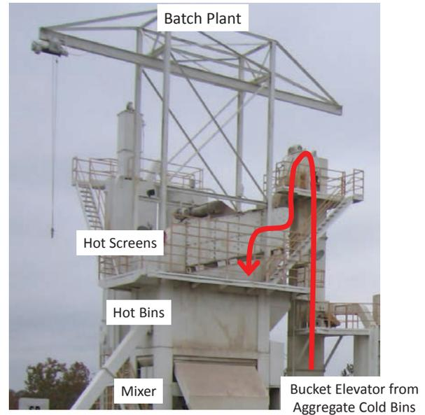
FIGURE 37 Components of a batch plant [Source: Stroup-Gardiner (2014)].
