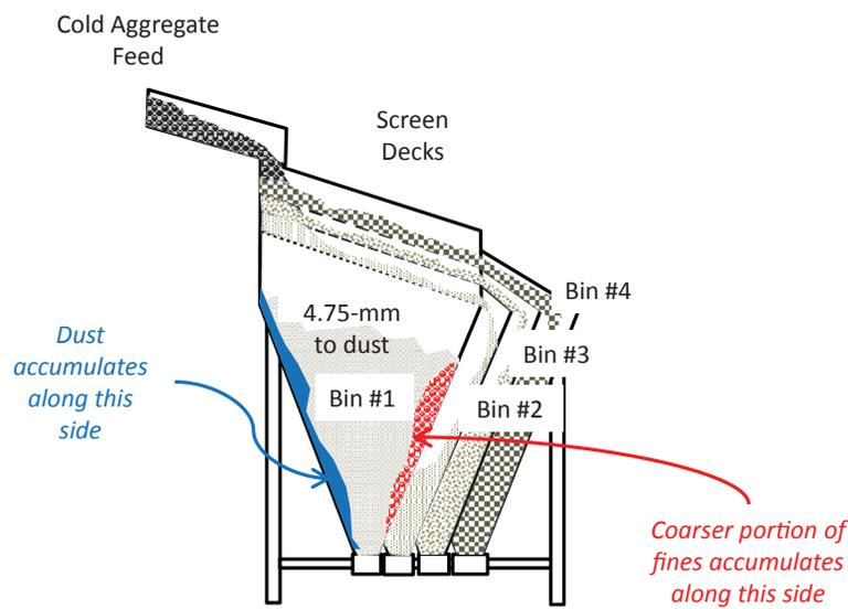
Aggregate segregation happens when the build-up of either dust or coarse aggregate gets too large and drops all at once into the mixer
