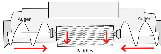
*Augers move mix from the outside of the windrow towards the paddles. The paddles rotate downward and push the mix onto the internal conveyor which deposits the mix into the paver hopper.*
