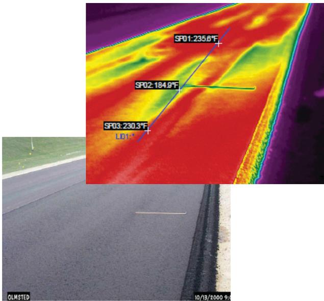
FIGURE 20 Temperature differences that reflect visible changes in texture (end-of-truck segregation) [Source: Adams et al. (2001)].
