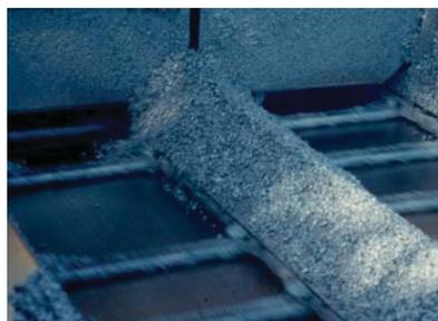
*Conventional drag slot configuration can fracture aggregate which shows up behind the screed as a coarser texture.*
