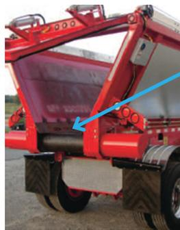
A conveyor belt in the bottom of the truck bed to move the mix out of the back of the truck.
