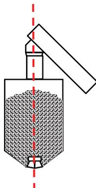
Chute not properly aligned over center of silo
