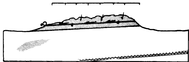
TYPE 6 SOFT PORTION OF SANDSTONE SEEPING OVER HARDER PORTION
