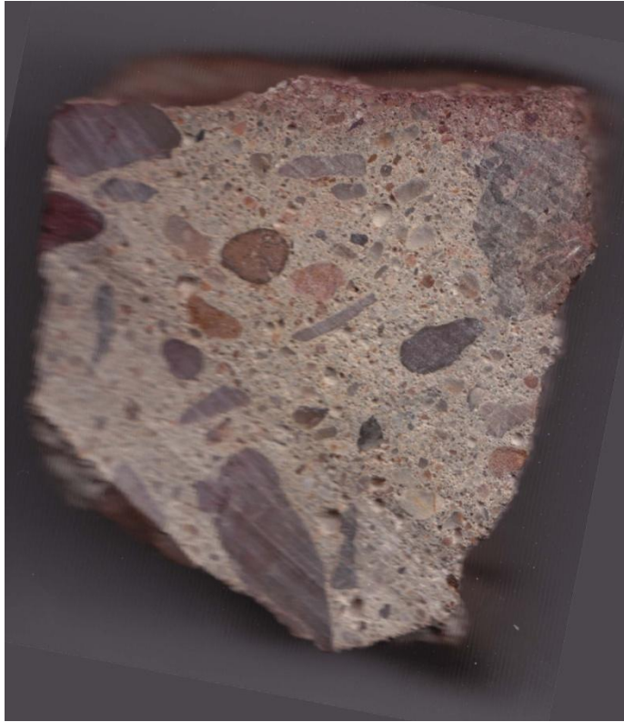
Figure 14: Stained Concrete Cross-Section
