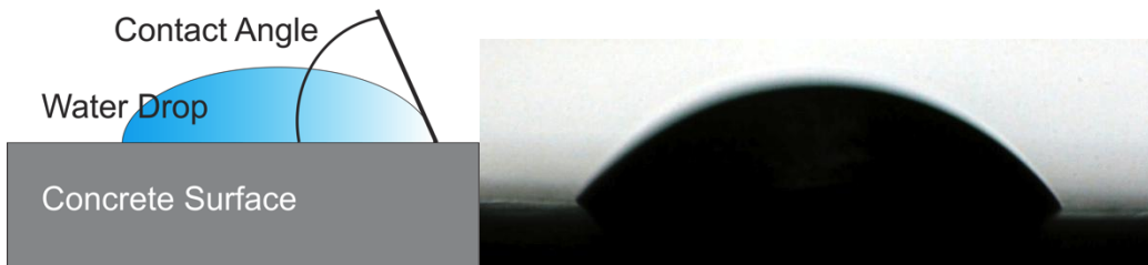
Figure 8: Graphical illustration of the contact angle and water droplet on glass.
