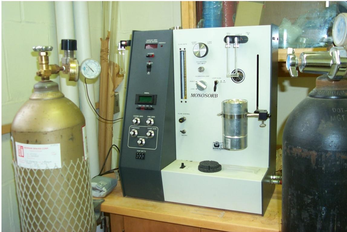
**Figure 3-4 Quantachrome MONOSORB<sup>®</sup> Apparatus for performing BET Analysis.**
