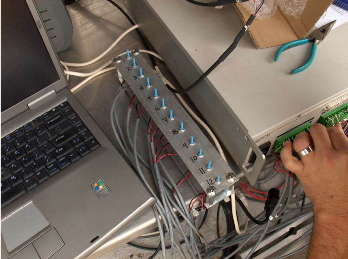
Figure 1. Twelve Channel Variable Resistor Array
