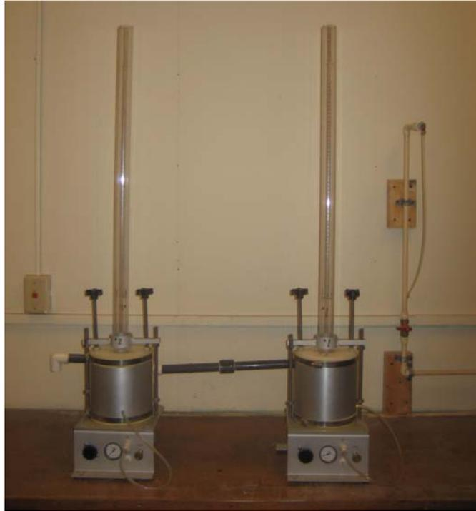
Figure 1 OSU's laboratory permeameters.
