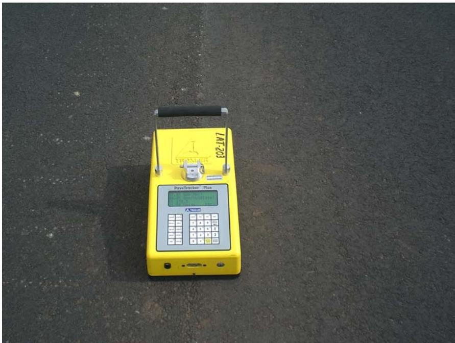
Figure 7 Electromagnetic gauge used for in-place density testing.
