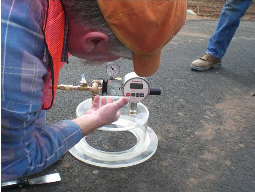
Figure 9 Measuring field permeability using the AIP.
