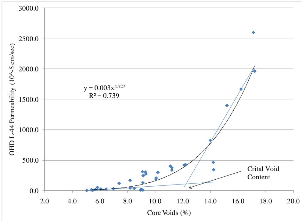
Figure 23 Critical void content for laboratory permeability.
