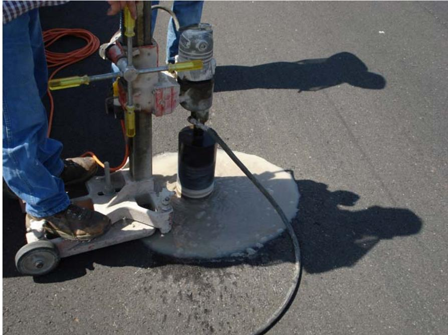
Figure 11 Obtaining field core for testing.
