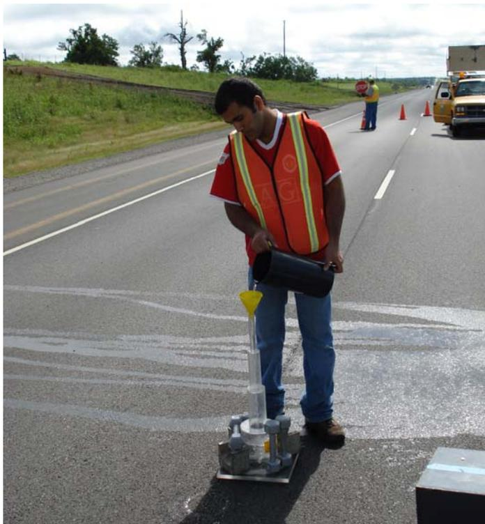
Figure 10 Measuring field permeability with NCAT permeameter.
