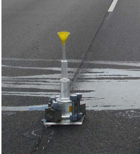
Figure 2 OSU's NCAT permeameter.
