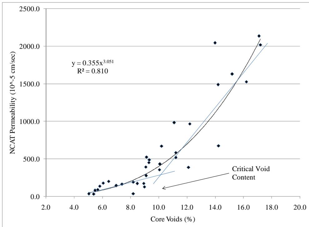
Figure 24 Critical void content for field permeability.
