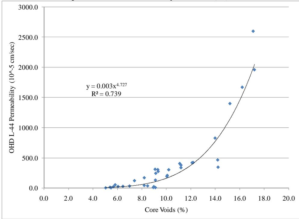
Figure 13 OHD L-44 permeability vs. core voids.
