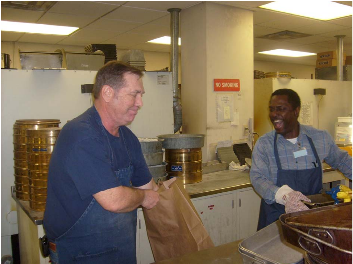
Figure 1. Ed Schratwieser (left) is extracting asphalt to run an aggregate gradation test while training Wilson Brewer (Anderson, 2007).
