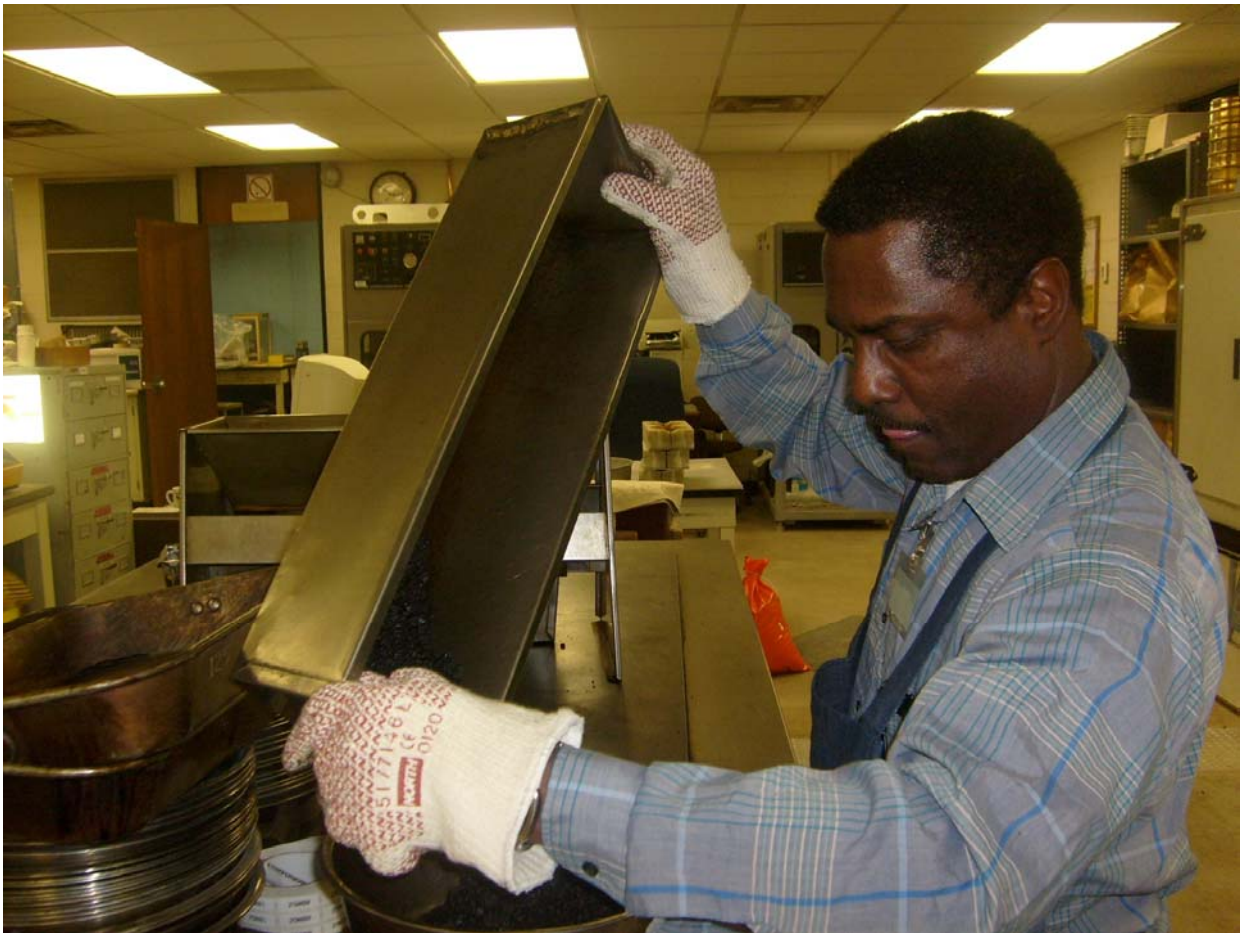
Figure 2. Wilson Brewer is measuring a specific amount of asphalt to run a laboratory molded specimen test (Anderson, 2007).
