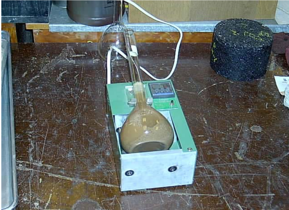
Figure 4. Langley fine aggregate de-airing device.
