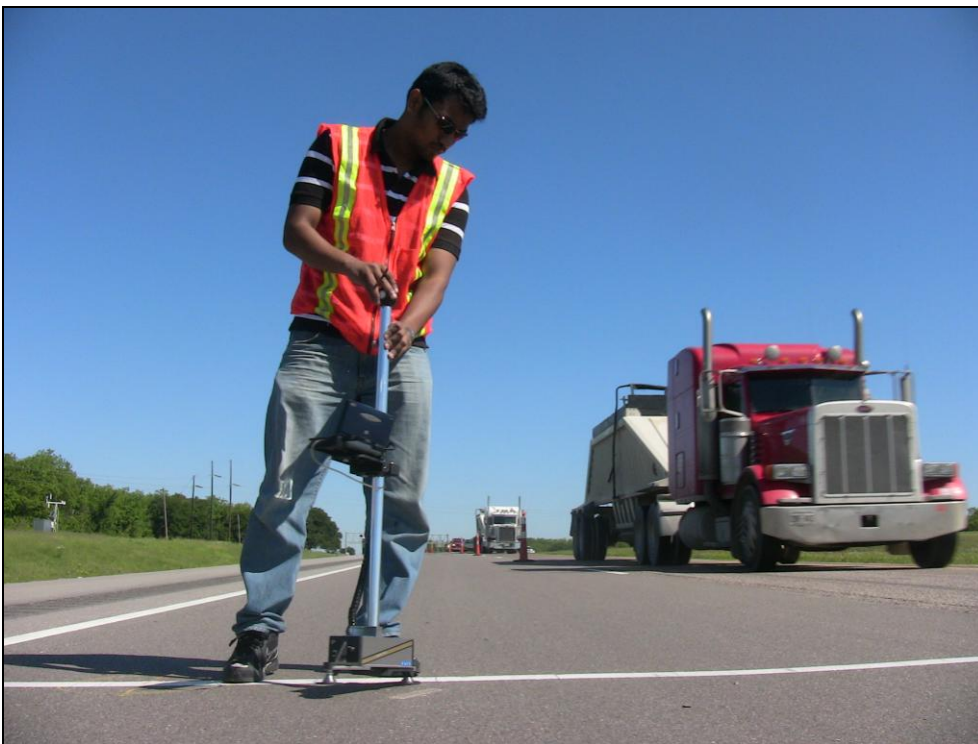
Figure 3: Rut Measurement with Face Dipstick®
