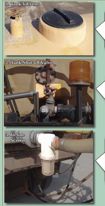
Sprayer tank holds the herbicide/water mixture and must be constructed with a material that is resistant to potential corrosion from certain herbicide formulations. There should be no leaks of tank contents anywhere.
