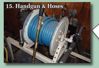
Handguns are used to make spot applications with high carrier rates (50 to 250 GPA, carrier rate is found on the herbicide label). Handguns should turn on and off consistently with no leakage. Hoses should be made of pressure rated materials resistant to bursting. Hoses should be checked regularly for cracks or aging and replaced before hose failure.
