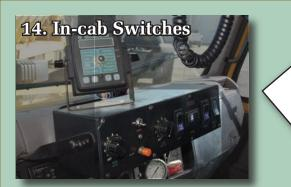
Switches turn spray solenoids on and off, activate control arms, and can control hydraulic motor speeds. All should function properly every time they are turned on or off. If the switch does not function properly every time, replace or repair it.
