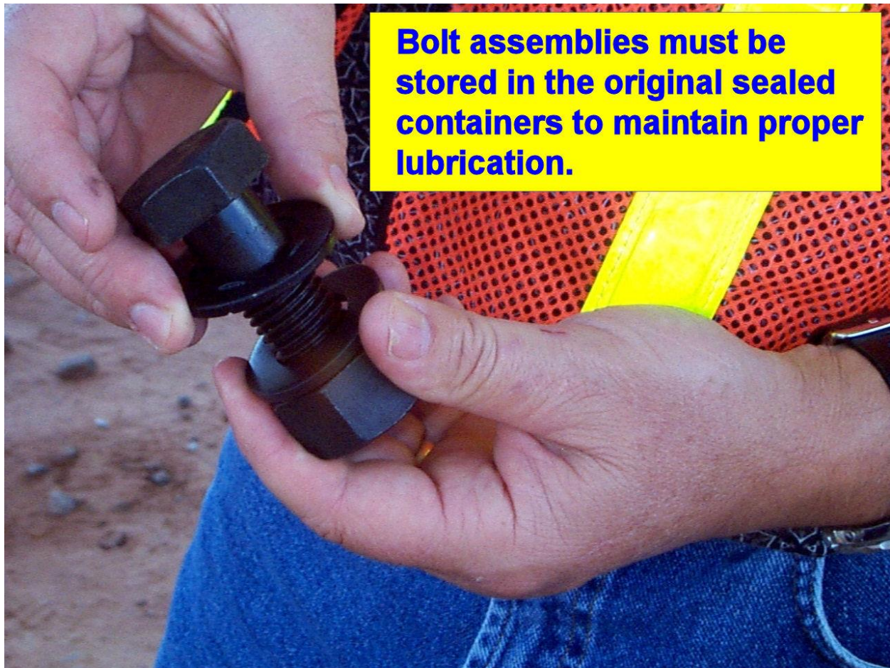
Figure 506:1. Photo. Proper Lubrication of Bolt Assemblies
