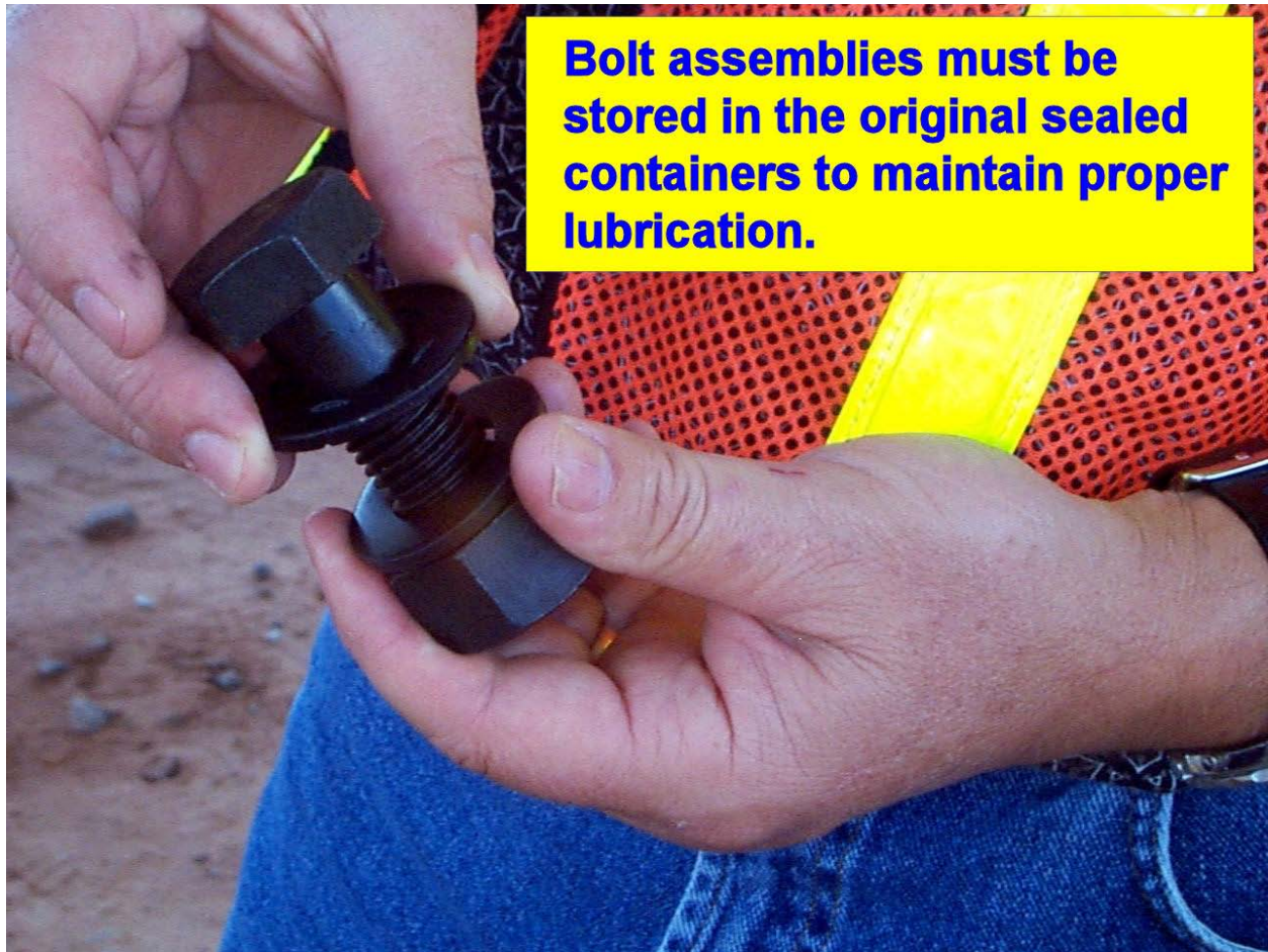
Figure 506:1. Photo. Proper Lubrication of Bolt Assemblies
