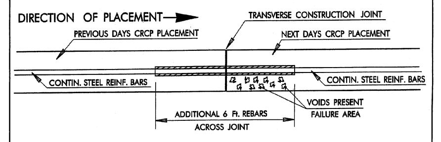
SOLUTION: Hand vibrate this area to ensure that the concrete placed above and below the steel reinforcement is thoroughly consolidated. Take test core(s) at each of these joint locations to inspect for this problem.
