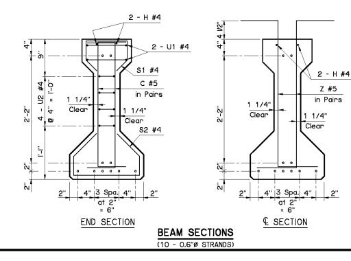
Information shown on this sheet is applicable only to the standard bridge cross-section with 40' Clear Roadway, 8" Deck Slab and 4 Beams at 11'-4" spacing. Any deviation requires custom design and details with an appropriate Dead Load Deflection Diagram.
