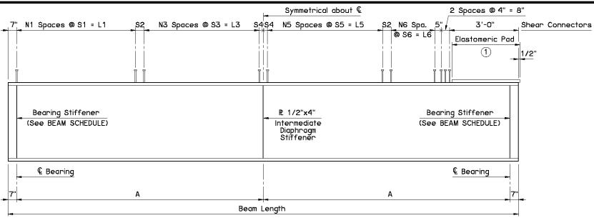
HALF ELEVATION AT ABUTMENT
