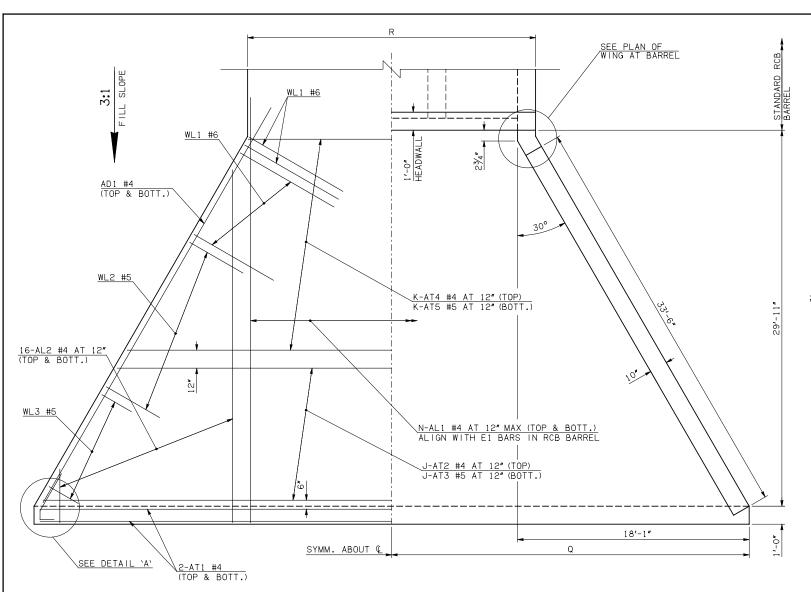
WINGWALL DIMENSIONS SPAN W D F 8' 12" 71/4" 31/2" 10' 12" 7\/4" 3\/2" 12' 12" 7\/4" 3\/2" 12' 12" 7\/4" 3\/2" 14' 12" 7\/4" 3\/2" 16' 13" 5\/4" 5\/4"
