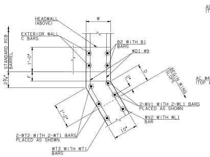
PLAN OF WING AT BARREL
