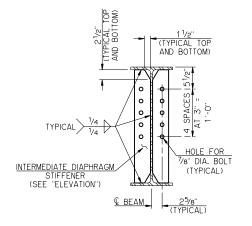
INTERMEDIATE DIAPHRAGM STIFFENER DETAIL
