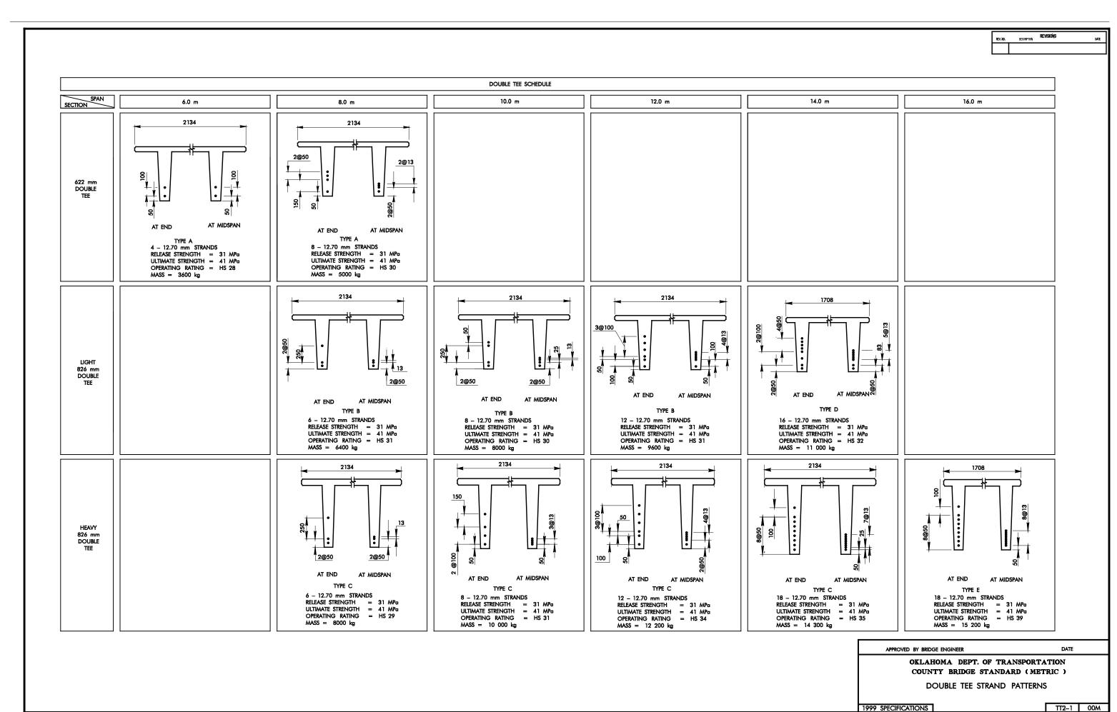
ALL DIMENSIONS ON THIS SHEET IN MILLIMETERS UNLESS OTHERWISE NOTED. CB-11M
