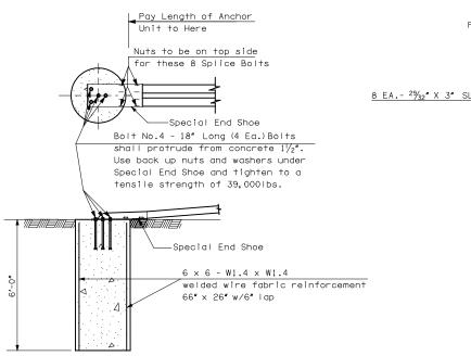
Class A Concrete to be placed into 30" Dia. hole to a depth of approx. 6'-0". Slope top of concrete to fit slope. Class A Concrete = 1.09 c.y.
