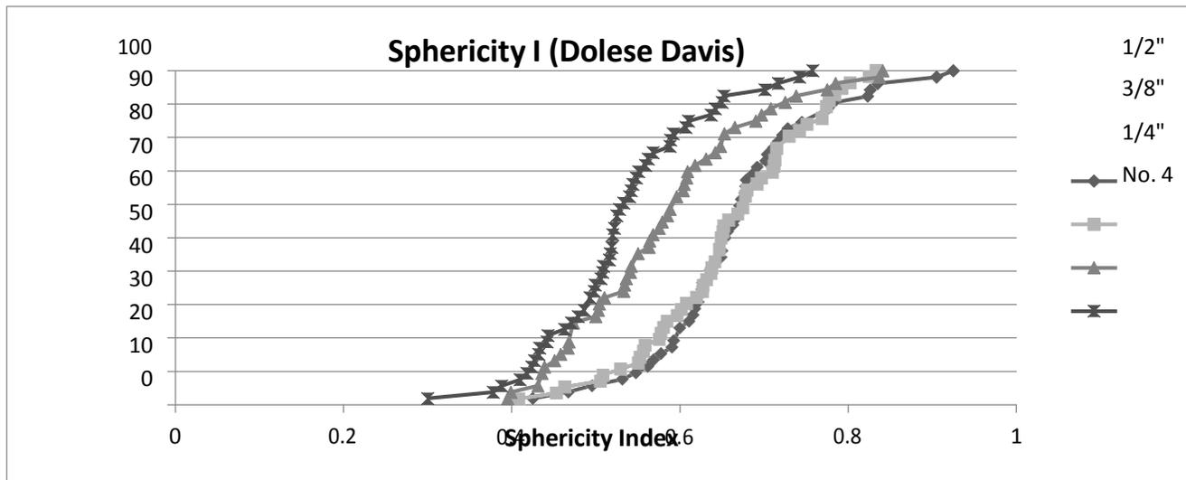
Figure 2 AIMS Output: Sphericity for Test Section Aggregate
