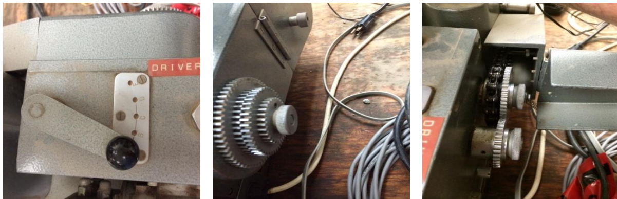
Figure 1. Clutch and gear rate adjustment
